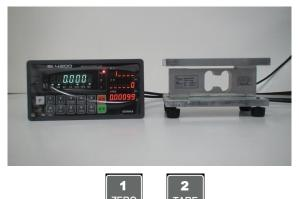
Before process "Unit Calibration", press TARE , and make display Weight is "ZERO". or
