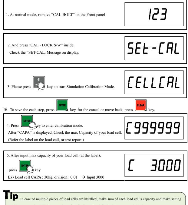
with max capacity. EX) There are 4pcs of load cells, and each load cell's Max capa is1,000kg.
