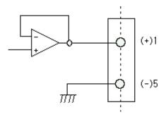
\* This Voltage output is proportioned on weight calibration and outputs 0~10V.
