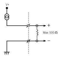
\* "LO" terminal is not a "GND", so this "LO" terminal do not be connected with other "GND" terminal on other devices.
